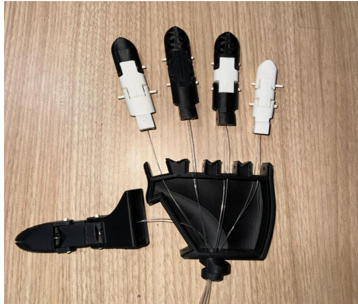
Fig.1. Physical Model of the Palm and Fingers with Fishing Lines as Tendons
